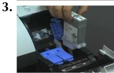
3. Place the appropriate color ink cartridge into machine as shown.
